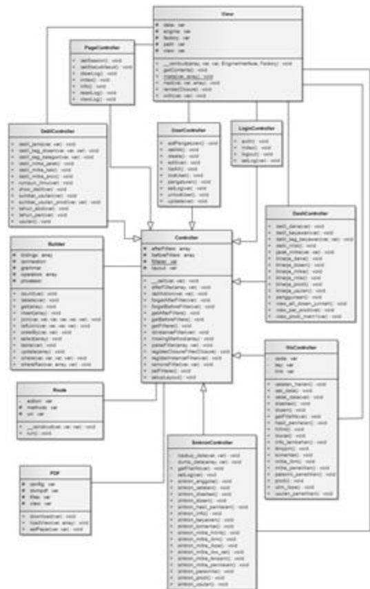
Gambar 5. Model Pengembangan MVC Dashboard PPM
