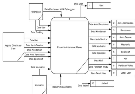
**Gambar 3** DFD level 0 Melakukan Proses Maintenance Master.
