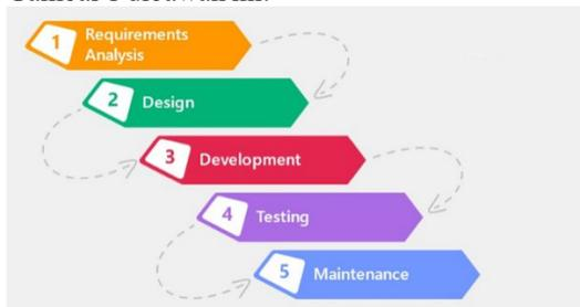
Gambar 1 SDLC Model Waterfall (Sumber: medium.com/purwanto, 2017)
