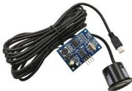
Gambar 3. Sensor jarak JSN-SR04T
