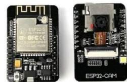
Gambar 3. ESP32-CAM
