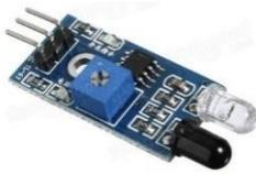
Gambar 4, Sensor IR Obstacle
