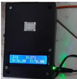
Gambar 8. Hasil tampilan Output LCD 16x2
