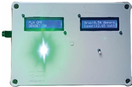
Gambar 6. Sensor tegangan Genset ON
