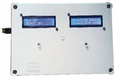
Gambar 7. Sensor tegangan Genset OFF
