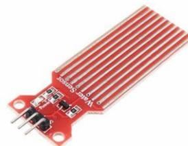
Gambar 3. *Hardware Sensor Water Level*
