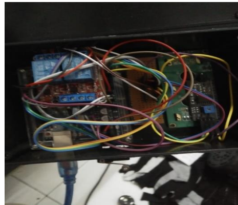
Gambar 5. Implementasi Arduino, Relay, LCD
